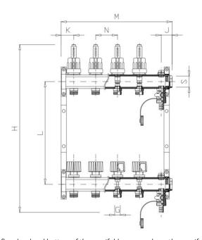
Recommended minimum installation clearances: 200mm between the finished floor level and bottom of the manifold. 100mm above the manifold, 50mm to either side of the manifold and allow and extra 100mm for the supply pipe work.
