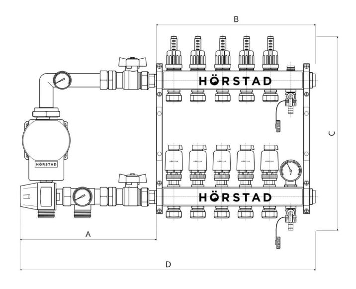
Recommended minimum installation clearances: 200mm between the finished floor level and bottom of the manifold. 100mm above the manifold, 50mm to either side of the manifold and allow and extra 100mm for the supply pipe work.
