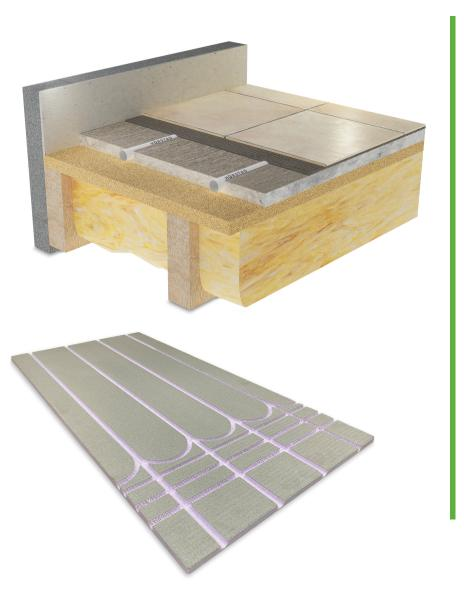
The routed overlay panels are manufactured from high density XPS which is thermally insulating, lightweight, waterproof and faced with a reinforced cement coating.
