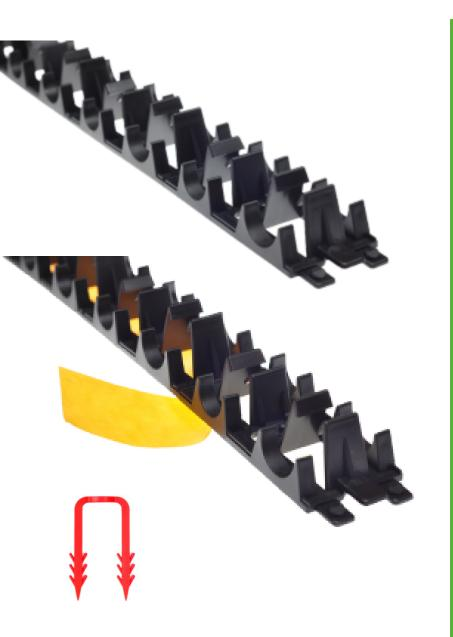
Clip Rail is used for wet underfloor heating and is great for use on large areas. Designed for pipes with diameters of 16-18 or 25mm. The rails are available in 1000mm lengths, consisting of two 500mm sections, 100 pieces per pack.
