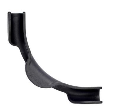
The pipe bends' support allows the installer to bend heating pipes in a 90 degree bow without forming kinks which impede flow within the pipe.
