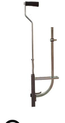
A Tacker Gun is an ergonomic device used for an effective fixing of underfloor heating pipe using tacker clips. The device has an appropriate adjustment system which protects the clips from falling out and allows to set the force of the arm returning to the base position.
