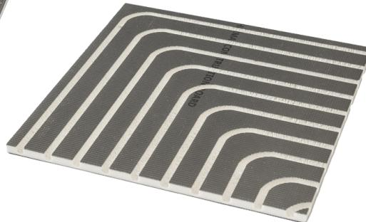
The routed overlay panels are manufactured from high density XPS which is thermally insulating, lightweight, waterproof and faced with a reinforced cement coating.
